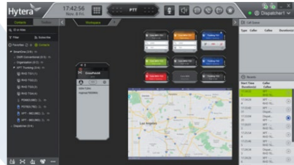
A Sample Dispatch Application Making and Monitoring Calls and Tracking User Locations
